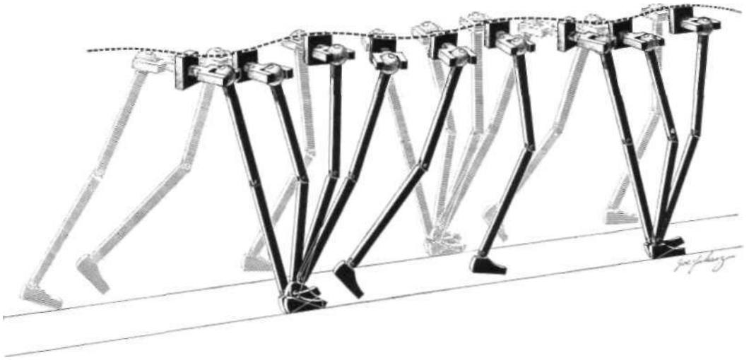
Fig. 8. The sum of the effects of the six determinants of gait. The pathway of the center of gravity is a smooth curve in both horizontal and vertical planes. From Saunders, Inman, and Eberhart (97), by permission of The Journal of Bone and Joint Surgery .
