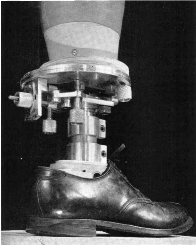
Fig. 15. Combination above-knee/below-knee adjustable leg in use as a trial below-knee prosthesis.
