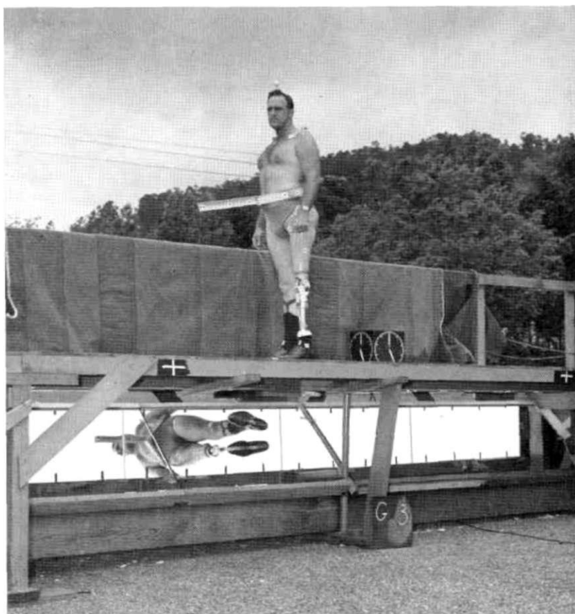
Fig. 1, The University of California glass walkway. With this device, motion pictures taken from a single camera yield sufficient information to determine relative motions of various segments of the body during level walking. Subject shown here is wearing an above-knee experimental leg.
