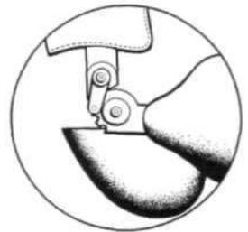
Fig. 12. Robin-Aids stump-actuated elbow lock.
